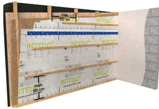
LEFT AND RIGHT: Fully sealed vapour and airtight layers Images: Ecological Building Systems
